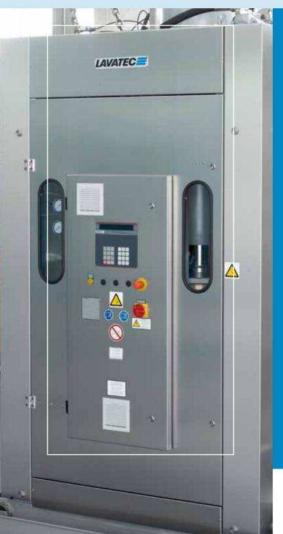
"The Lavatec Water Extraction Press ensures that the dryers downstream need to evaporize smaller amounts of water."
